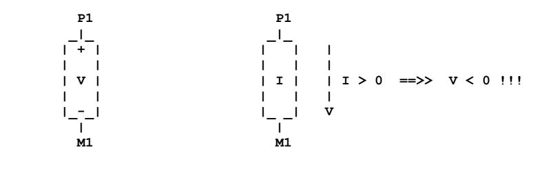
[V, id, P1, M1]; voltage source [I, id, P1, M1]; current source
