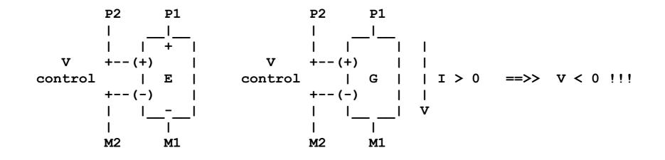
[E, id, P1, M1, P2, M2]; voltage controlled voltage source [G, id, P1, M1, P2, M2]; voltage controlled current source
