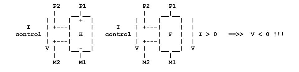
[H, id, P1, M1, P2, M2]; current controlled voltage source [F, id, P1, M1, P2, M2]; current controlled current source
