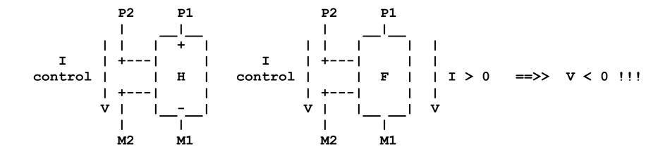
[ H, id, P1, M1, P2, M2 ]; current controlled voltage source [ F, id, P1, M1, P2, M2 ]; current controlled current source
