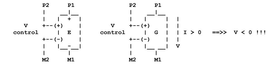
[ E, id, P1, M1, P2, M2 ]; voltage controlled voltage source [ G, id, P1, M1, P2, M2 ]; voltage controlled current source
