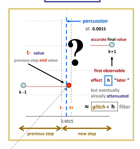
warning: in rubmode ( when no explicit NAPA delay ) the overall simulation waveform appears just shifted in time
